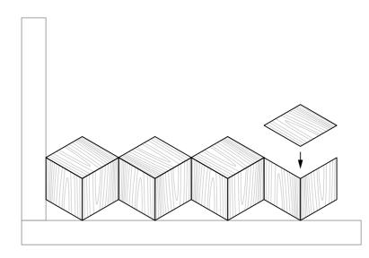
Install the second row, placing the tiles horizontally. Make sure the wood grain runs in the same direction across the whole row (e.g. diagonally down).
