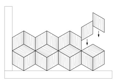
Install the third row similarly to the first, with the wood grain running vertically on all tiles.
