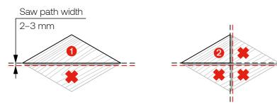
Use a fine-toothed hand saw to cut the edge tiles, then sand the sawn edges with a sanding block or sandpaper.
