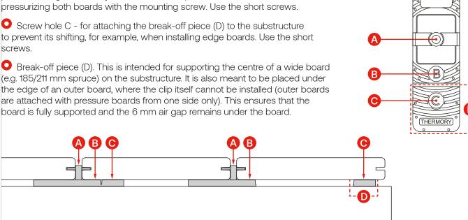
Since the boards are attached using only a pressure plate, the mounting screw should be tightened only when both boards resting on the clip are in place, i.e. both ends of the pressure plate are in the grooves of the boards. When tightening the mounting screws, you must use the medium setting on the drill so that the screw does not go too deep into the screw hole. If the screw is driven too forcefully into the pressure plate, the tension on plate will give way.
