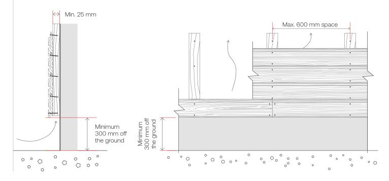
Installation guide Cladding Boards
