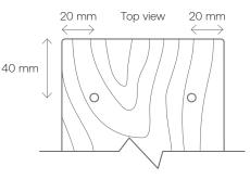
The length of screws or nails should be at least 2.5 times the thickness of the board at its thickest point.
