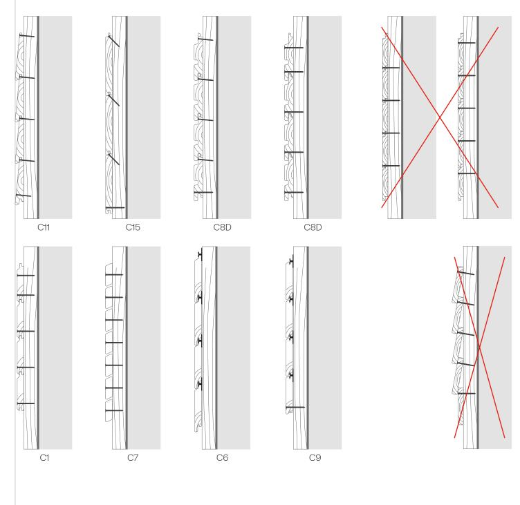
For shiplap profiles, leave an air circulation space of 2-3 mm to allow for swelling of the wooden boards.
