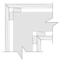
Cut the boards to a 45-degree angle.
